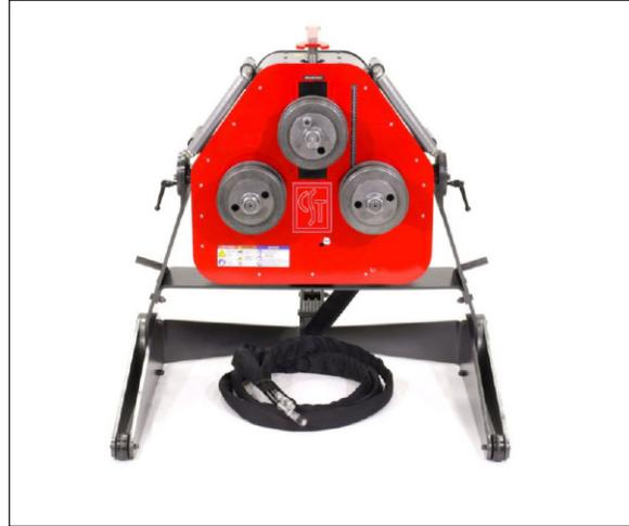
Designed for medium to heavy material, the Radius Roller powers through your job quickly and accurately. Roll rod, flat, angle and channel. The variable speed, hydraulic drive allows you to "dial in" the appropriate speed for various materials. Quickly change the orientation from vertical for smaller projects to horizontal for those larger, heavier jobs.
