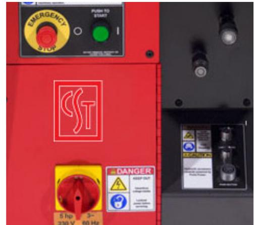
If the machine fails to cycle, power down the Porta-Power by depressing the red button on the starterbox, consult the trouble shooting section of the manual.
