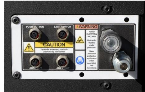
Factory Installed Ironworker Hydraulic Accessory Pack
