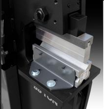
Controlled, repeatable bends in 1/4" thick mild steel
