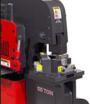
Load 3 different pipe notcher dies at once and quickly switch from one size to the next Up to 2" Schedule 40 pipe (requires dies)
