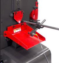
Adjustable proximity switch automates production when cutting repeatable lengths
