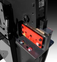
Reduce deformation in 1/4" to 1" mild steel rod
