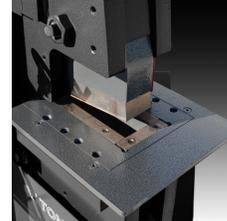
Precisely notch plate or angle up to 2" mild steel
