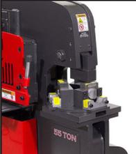
Load 3 different pipe notcher dies at once and quickly switch from one size to the next Up to 2" Schedule 40 pipe (requires dies)
