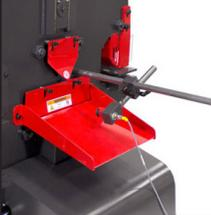
Adjustable proximity switch automates production when cutting repeatable lengths
