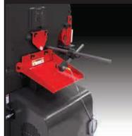
Adjustable proximity switch automates material cutting to repeatable lengths
