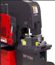
Load 3 different pipe notcher dies at once and quickly switch from one size to the next Up to 2" Schedule 40 pipe (requires dies)
