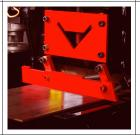
Flat Bar Shear 3/8" x 24" 1/2" x 14" 1" x 4" mild Steel
