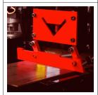
Flat Bar Shear 3/8" x 14" 1/2" x 12" 3/4" x 4" mild Steel
