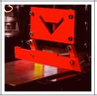
Flat Bar Shear 1/2" x 18" 3/4" x 14" 1" x 10" mild Steel
